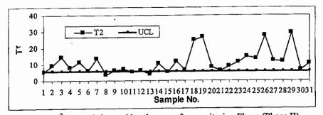
Fig. 18 T<sup>2</sup> Control chart with subgroups for monitoring Phase (Phase II).
