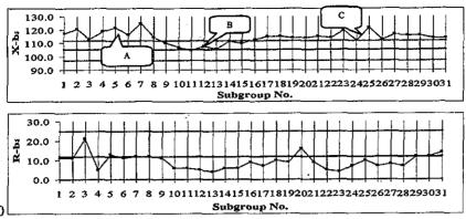
Fig. 4 X bar-R charts  $T_{bwi}$  by subgroup -monitoring Phase. UCLx = 111.75, CLx = 104.98, LCLx = 97.21; UCLr = 24.82, CLr = 11.76, LCLr = 0.0
