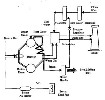
Fig. 1 Schematic diagram of boiler steam generation.
