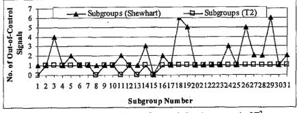
Fig. 22 Comparison of out-of-control signal generated of T<sup>2</sup> and Shewhart control charts with subgroups.
