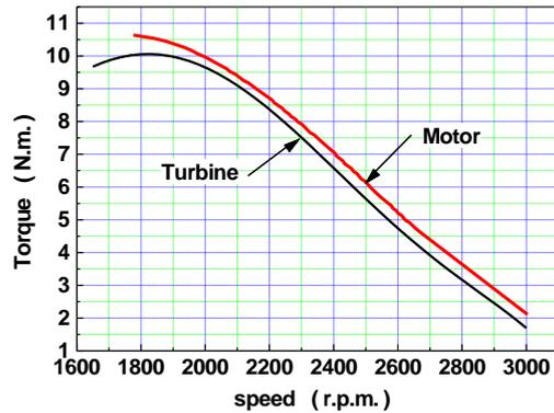
Fig. (8) Turbine torque and motor torque versus the rotor speed for adding resistance.
