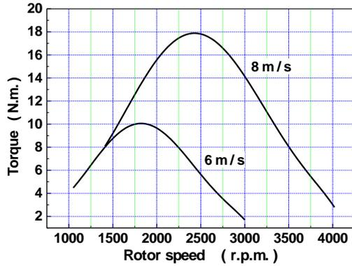
Fig. (1) Turbine torque variation with speed after gear box
