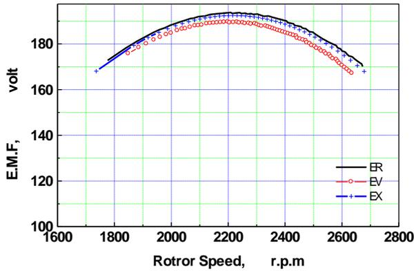
Fig. (15) Induced e.m.f.-speed characteristics for voltage, resistance and reactance variation.
