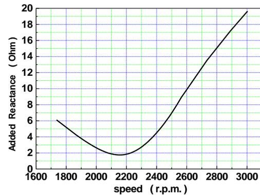
Fig.(7) Added reactance versus the rotor speed
