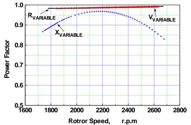
Fig. (14) Power factor-speed characteristics for voltage, resistance and reactance variation.
