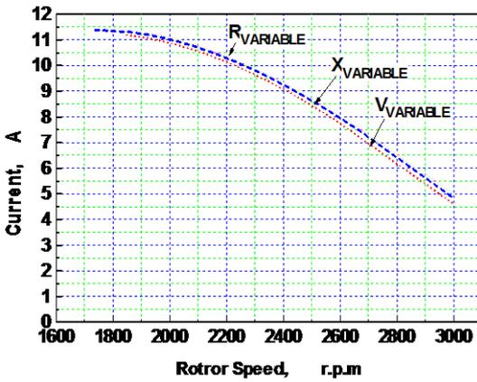
Fig. (11) Motor current-rotor speed characteristics for voltage, resistance and reactance variation.
