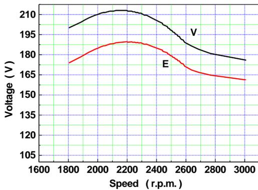
Fig. (5) The variation of the terminal voltage with rotor speed.
