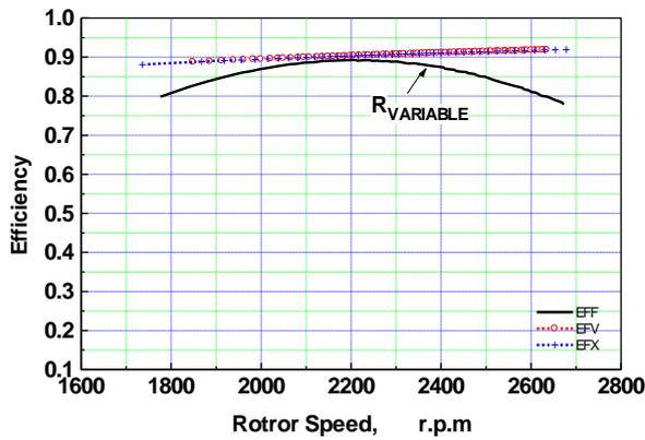
Fig. (16) Efficiency-speed characteristics for voltage, resistance and reactance variation.
