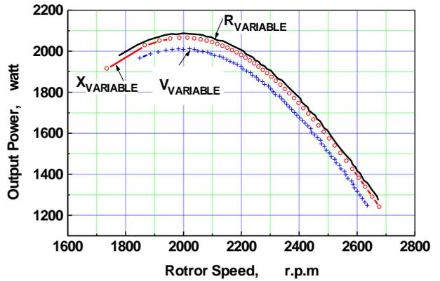
Fig. (13) Output power -speed characteristics for voltage, resistance and reactance variation.
