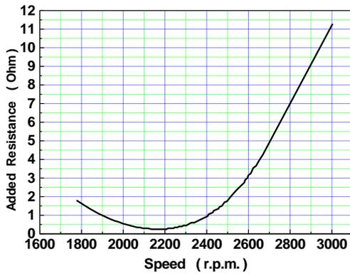
Fig.(9) Added resistance versus the rotor speed.
