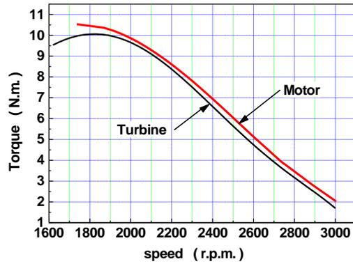
Fig. (6) Turbine torque and motor torque versus rotor speed with adding external reactance.
