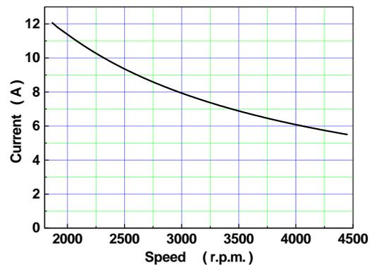
Fig. (3) Motor current variation with rotor speed
