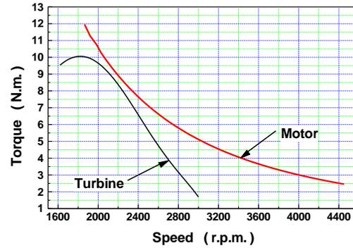
Fig. (2) Turbine torque / speed curve and uncontrolled motor torque / speed curve.
