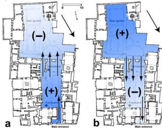
Figure 2: Al- Suhaymi house garden and the recommended air circulation according to the difference in pressure air [Source: [1]]
