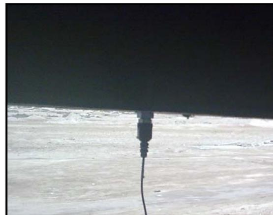
Fig. 7 Photo of one of the installed accelerometers
