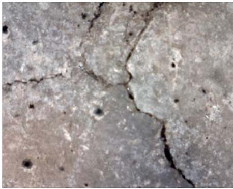
Fig. 8 Severe cracking at 750 °C
