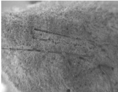
**Fig. 6** The beds of melted PP fibers at 400°C
