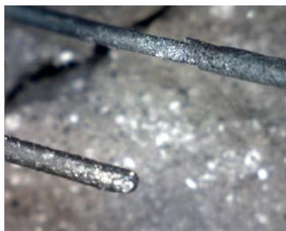
**Fig. 7** Oxidation of SF at 600°C
