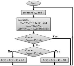
Fig. 16. Flow chart of temperature measurement based MPPT technique.
