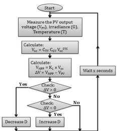
Fig. 6. Flow chart of Modified fractional open circuit voltage technique.
