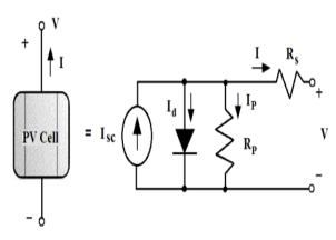
Fig. 2. Equivalent circuit of a PV cell using the single exponential model.
