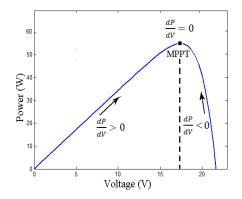
Fig. 10. The power-voltage characteristics of a PV panel.
