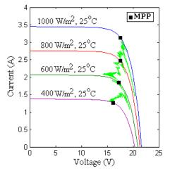
Fig. 12. Tracing of MPP using IncCond technique.
