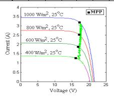
Fig. 15. Tracing of MPP using FLC based MPPT technique.
