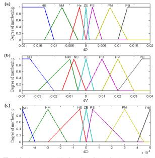
**Fig. 14.** The membership function of (a) The input variable  $\Delta P$ ; (b) The input variable  $\Delta V$ ; (c) The output variable  $\Delta D$ .
