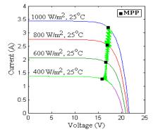
Fig. 7. Tracing of MPP using modified open circuit voltage technique.
