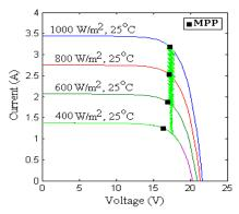
Fig. 17. Tracing of MPP using temperature measurement based MPPT technique.
