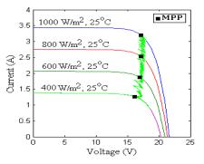
Fig. 9. Tracing of MPP using P&O technique.
