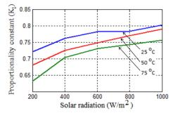
Fig. 5.  $V_{MPP}$  as a percentage of  $V_{OC}$  as functions of irradiance and temperature.
