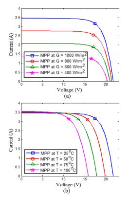
**Fig. 3.** Simulated I-V curves of a specific solar module, SM55, (a) at different irradiance at 25 <sup>o</sup>C, (b) at different temperature at 1000 W/m<sup>2</sup>.
