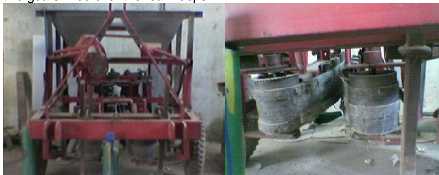
a-View of application points and 3 forming furrows' spacing b-View of ply rolling and Pulling belt (harvester unit) Fig. 14: Photo of (planting and harvesting) sugar beet machine
