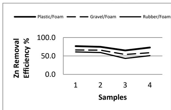
**Fig. (6)** Removal Efficiency of Zn(II) after mixing the media with polystyrene
