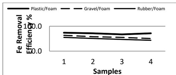
Fig. (12) Removal Efficiency of Fe(III) after mixing the media with polystyrene.
