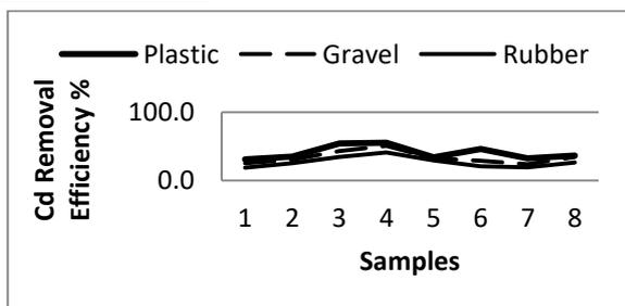
Fig. (13) Removal Efficiency of Cd(I) before mixing the media with polystyrene.
