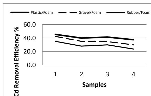
Fig. (14) Removal Efficiency of Cd(II) after mixing the media with polystyrene.
