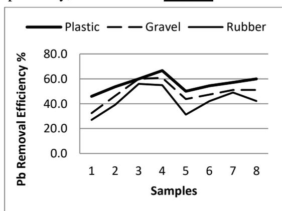
**Fig. (7)** Removal Efficiency of Pb(II) before mixing the media with polystyrene.
