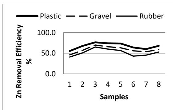
**Fig. (5)** Removal Efficiency of Zn(II) before mixing the media with polystyrene
