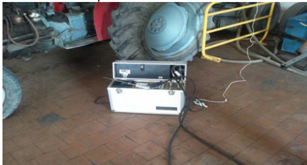
Fig. 2: The exhaust gas analyzer
