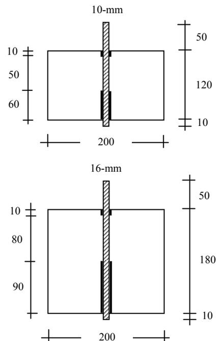
Figure 3. Configuration of push-out bond test specimens
