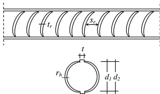
Figure 2. Geometry of the steel bars
