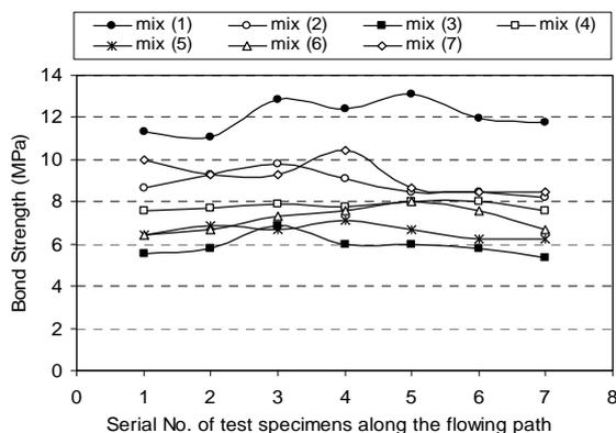
Figure 7. Bond strength along the flowing path (16-mm bar diameter specimens)
