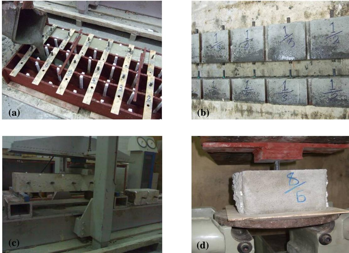
Figure 4. Preparation and testing of push-out test specimens
