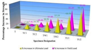
**Fig. 18:** Effect of GFRP plating on strength for t-series beams [33].
