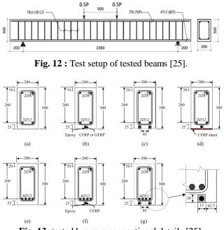
Fig. 13: tested beams cross sectional details [25].
