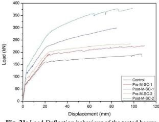
**Fig. 21:** Load-Deflection behaviour of the tested beams [37].
