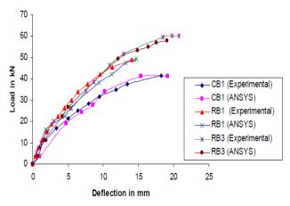
Fig. 4: Experimental and FEM load-deflection curves for beams [18].
