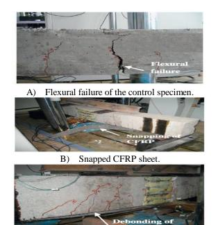
CFRP C) CFRP debonding from mid-Span.
