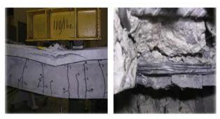
A) Concrete crushing B) FRP rupture Fig. 10: Failure modes of strengthened RC beams using NSM technique [23].
