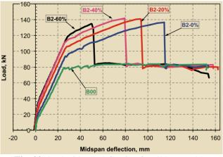
Fig. 20: load midspan deflection for all beams [34].
