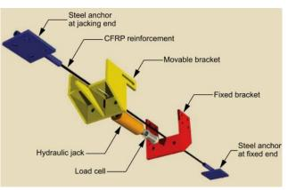
Fig. 19: Components of prestressing system [34].
