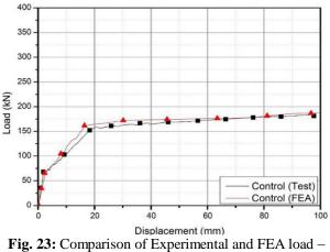
**Fig. 23:** Comparison of Experimental and FEA load - deflection curve for control beam [37].
