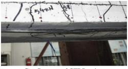
C) Rupture of CFRP strips.
