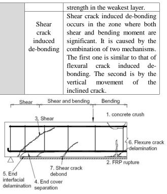
Fig. 3: Failure modes of EB strengthened beams [17].
