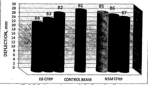
Fig. 7: Deflection versus beam type plot for all strengthened beams
