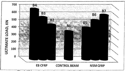
Fig. 6: Ultimate load versus beam type plot for all strengthened beams
