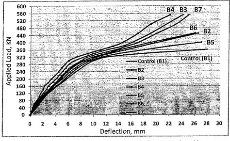
Fig. 5: Load versus mid-span deflection plot for all the strengthened beams
