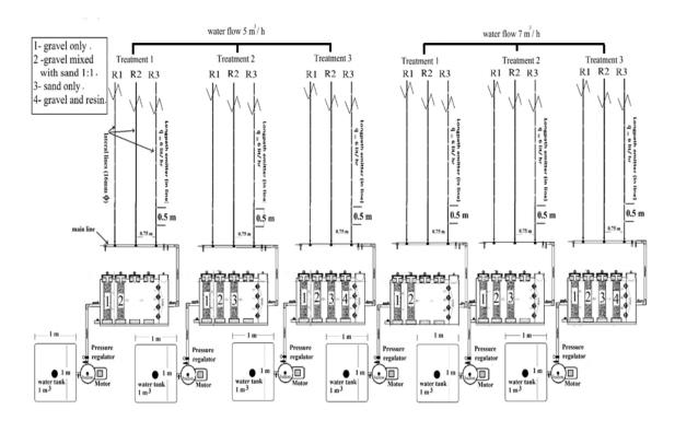
Fig (6): A schematic diagram of the tested treatments for both Nile and mixed agricultural drainage water under 5 and 7 m<sup>3</sup>.h<sup>-1</sup> of water flow rate inside the new filter (6 treatments for each type of water).
