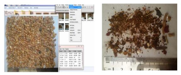
Fig. (7): Image Java Windows program used to measure grain media size and deposits before and after filtration process.
