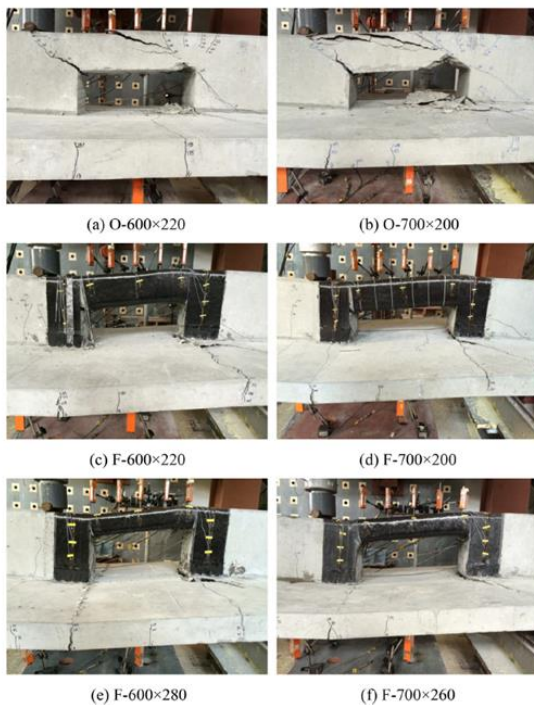
Figure 12: Failure modes of test specimens [38]
