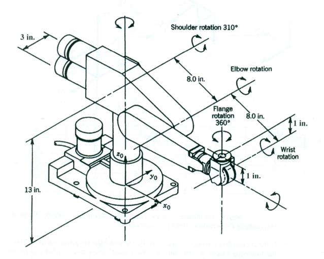
To derive the forward kinematic equations, the following coordinates frames and links parameters are suggested.
