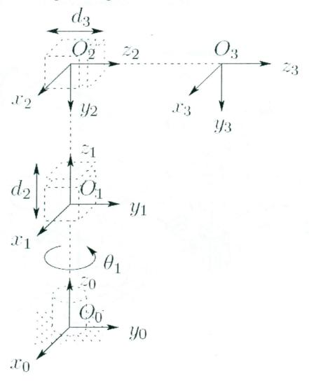
4. Derive the Euler-Lagrange equations for the cylindrical manipulator shown above assuming that the moments of inertia of all links are zero and the mass of each link equals 1. Let the centers of masses of links 1, 2, and 3 coincide with  $O_1$ ,  $O_2$ , and  $O_3$  respectively.
