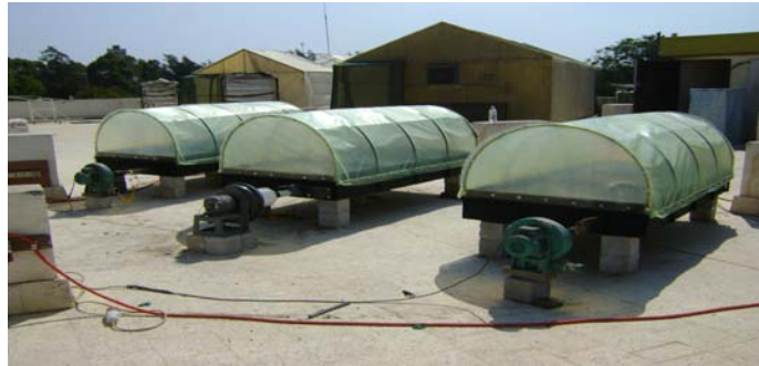
Fig. (1): Solar tunnel greenhouses (Quonset type) used as an active solar dryers during the experimental period.
