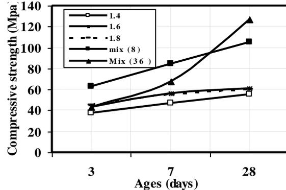
Figure (8) Effect of Dolomite-Sand ratios on the Compressive Strength using 0.5 % Superplasticizers
