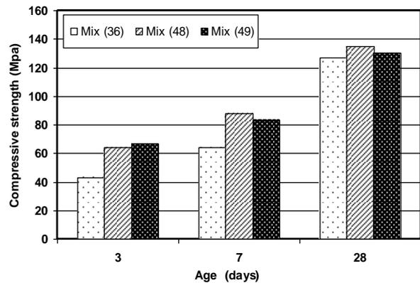
Figure (12) Effect of Steel Fibers on the Compressive Strength
