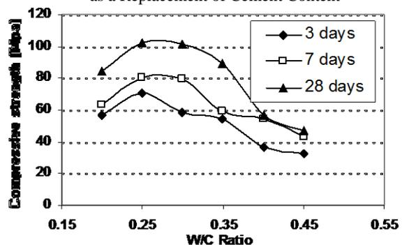
Figure (2) Relationship between the Compressive Strength and Water / Cement Ratio at 15% of Silica fume as a Replacement of Cement Content
