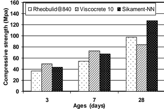
Figure (6) Effect type of superplasticizers on the compressive strength at Water-Cement ratio 0.3
