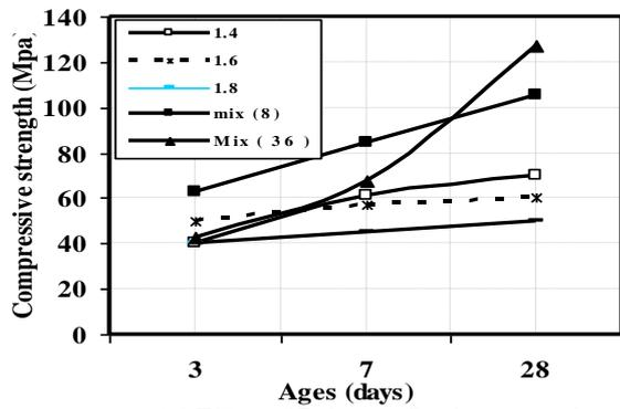
Figure (7) Effect of Dolomite-Sand ratios on the Compressive Strength without Superplasticizers
