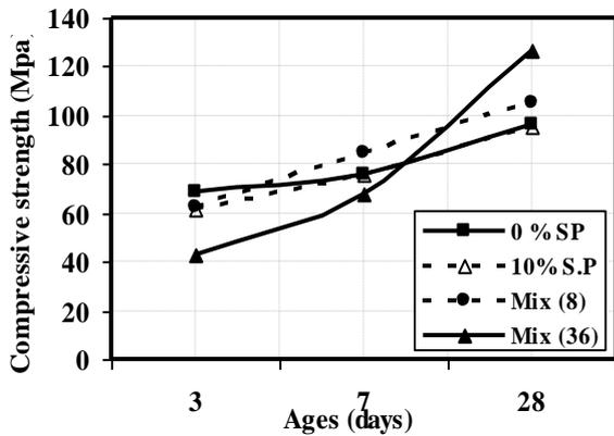
Figure (9) Effect of Quartz Powder on the Compressive Strength.
