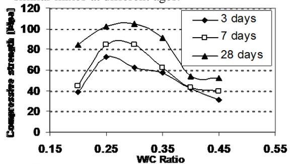
Figure (1) Relationship between the Compressive Strength and Water / Cement Ratio at 10% of silica fume as a Replacement of Cement Content
