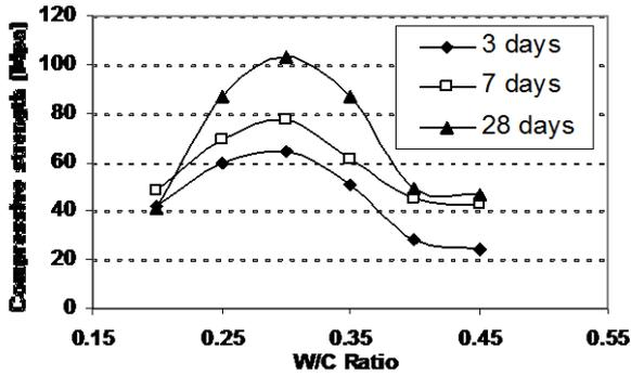
Figure (3) Relationship between the Compressive Strength and Water / Cement Ratio at 20% of Silica Fume as a Replacement of Cement Content
