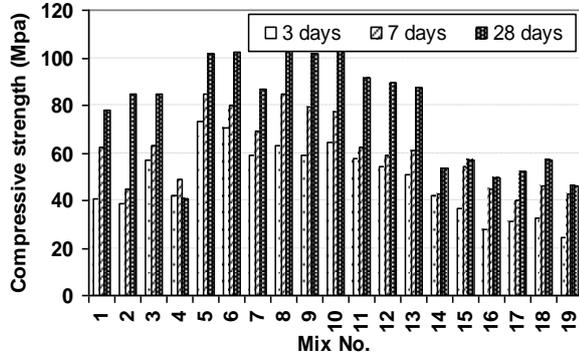
Figure (5) Relationship between the Mix No. and the Compressive Strength for the Mixes Contain different Percentages of Silica Fume Mixes without Superplasticizer
