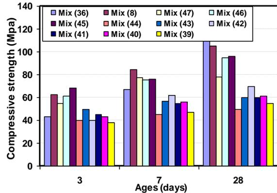
Figure (11) Comparison between the Compressive Strength and the Ages for the Concrete Mixes Contained different Types of Aggregates
