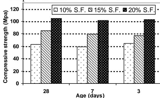
Figure (4) Relationship between the Compressive Strength of Different Percentages of Silica Fume as a Replacement of Cement Content at 0.3 W/C Ratios.
