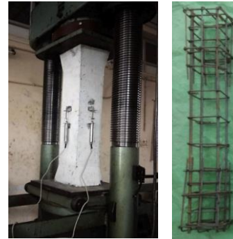
Figure 20: Test setup and specimen details [106]
